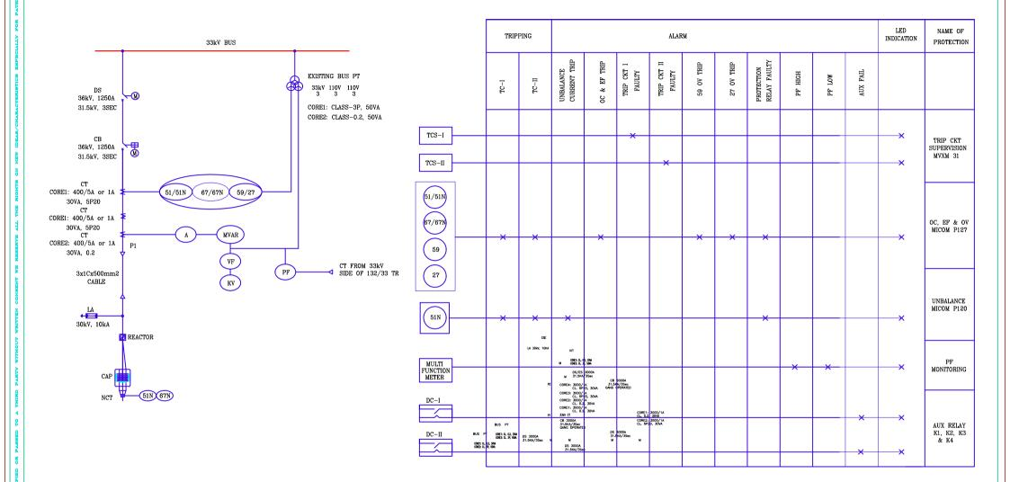
\*\* Timer based lockout relay has to be provided in CB for safe discharge of capacitor bank.
