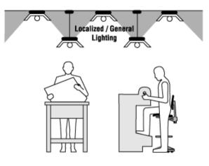
Local (or task) lighting increases light levels over the work and immediate surroundings. Local lighting often allows the user to adjust and control lighting and provides flexibility for each user.
