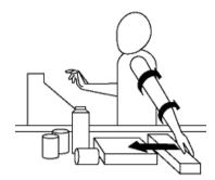
Figure 3C - Hazardous reaching movements - reaching behind the trunk
