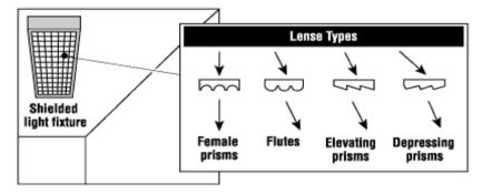
Louvers are baffles that shield the bulb from view and reflect light. The baffles can be contoured to control light and decrease brightness. Parabolic louvers are specially shaped grids that concentrate and distribute light.
