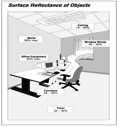
In addition, light fixtures that are too widely spaced or wrongly positioned can create shadows. Objects between the light fixture and work being done can block the light and cast shadows. Likewise, workers sitting with their backs to windows, with light fixtures directly overhead or to the rear, cast shadows on their own work surfaces.
