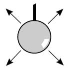
**Indirect light fixtures** distribute 90 to 100 percent of the light upward. The ceiling and upper walls must be clean and highly reflective to allow the light to reach the work area. They provide the most even illumination of all the types of fixtures and the least direct glare. Indirect light fixtures are usually used in offices.
