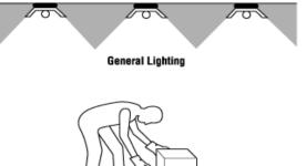
Localized-general lighting uses overhead fixtures in addition to ceiling fixtures to increase lighting levels for particular tasks.
